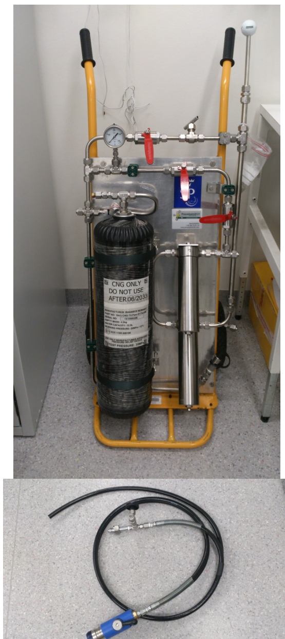
Figure 1: Modified sampler with a union-tee-connection to rinse the spray nozzle (top) and device to flush the buffer-tank with nitrogen (bottom)
